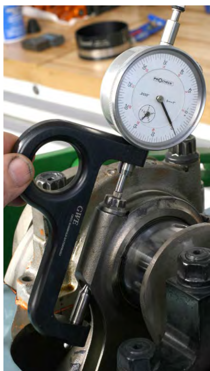
Without disturbing the gauge dial, place the gauge on the torqued bolt to read stretch.
