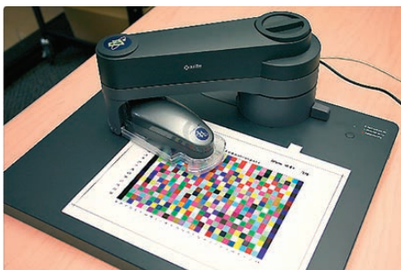
Figure 5. A color target document consisting of swatches of a full range of colors is printed to the specific substrate and then scanned with the device.
